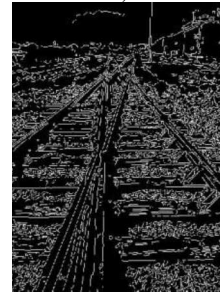
Fig. 11 Performing feature extraction by applying edge extraction on the image
