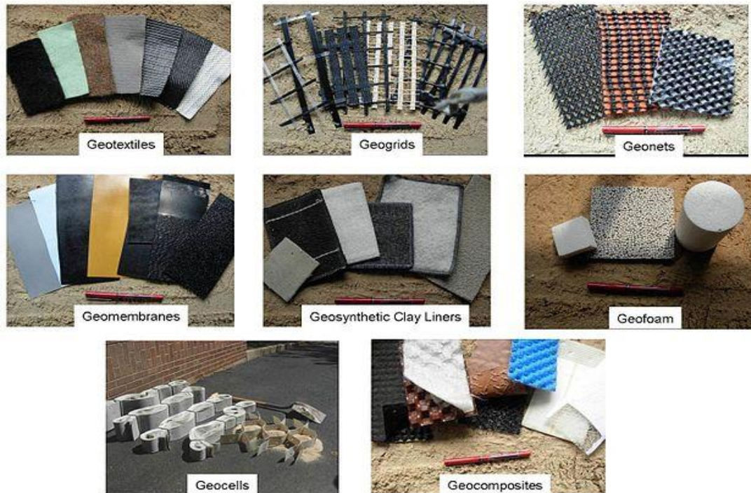
Figure 1. Types of Geosynthetic Materials [1]
