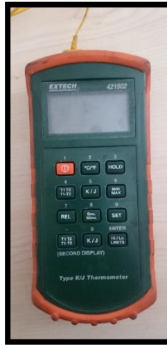
Şekil 7.4. Extech Instruments 421502 Model K/J tipi termometre
