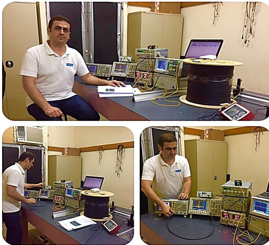
Figure 4.9-B: Practically at working in Laboratory RoF Using Fiber Cable (2km, 10m, 9m, and 3m).
