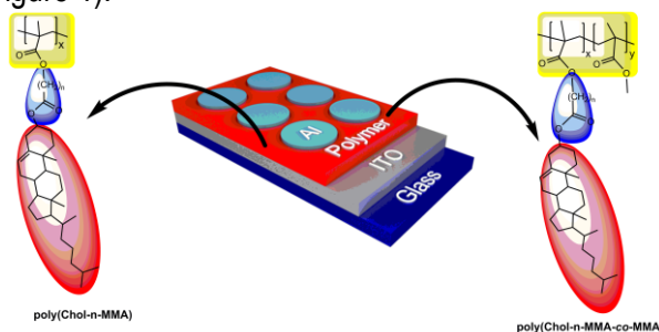
Figure 1. Design schematic of parallel plate structure and methacrylate-based polymers used for impedance spectroscopic analysis
