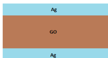
Fig. 1. Illustration for the device fabrication.
