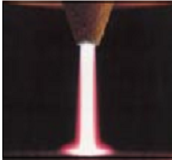
Şekil 3.14. Plazma transfer ark alevi (Gür, 2009)
