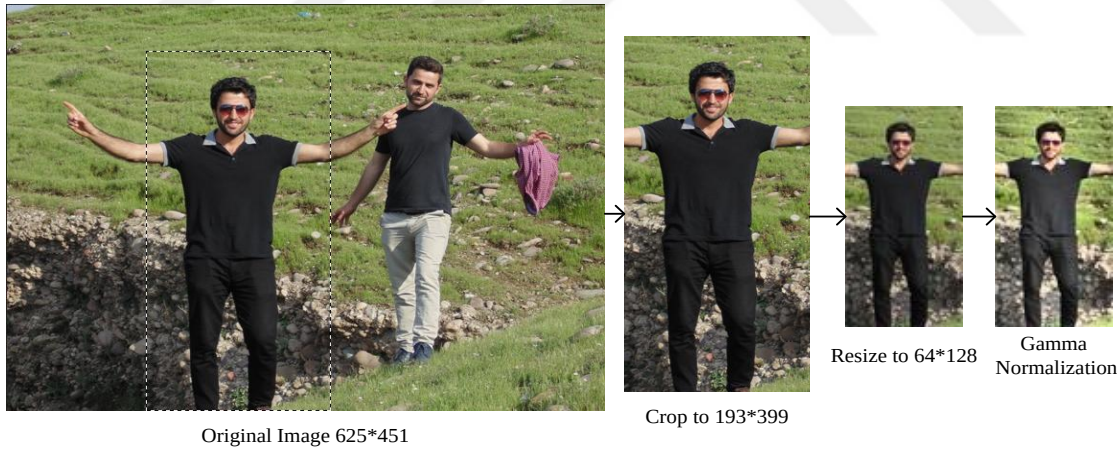
Figure 5.2. Preprocessing image and gamma normalization
