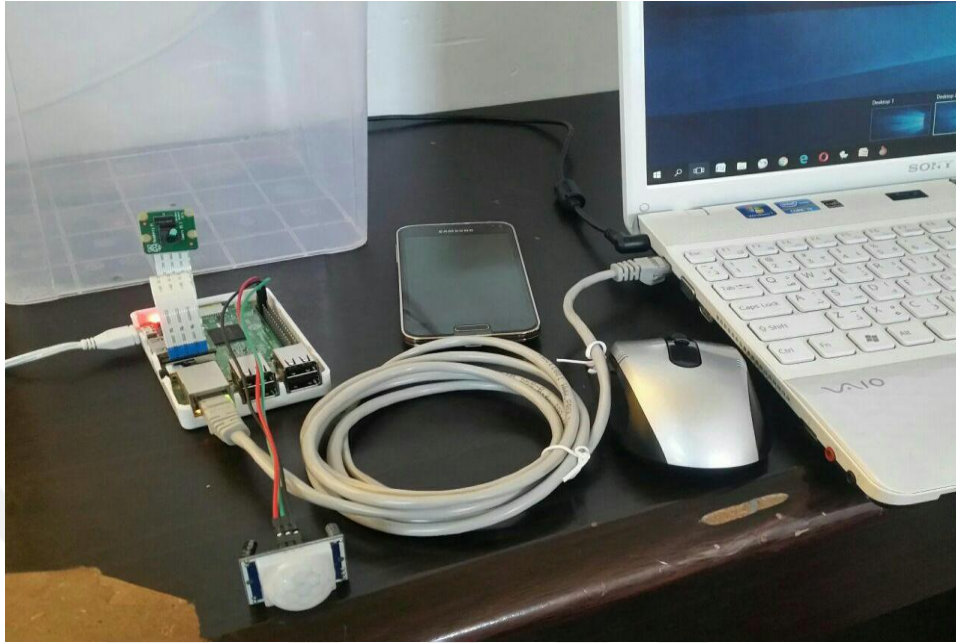
Figure 3.6. Experimental setup for face detection application
