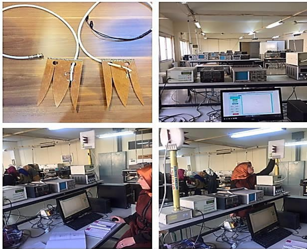
Figure 4.2: Setup for Radiation Pattern Measurements
