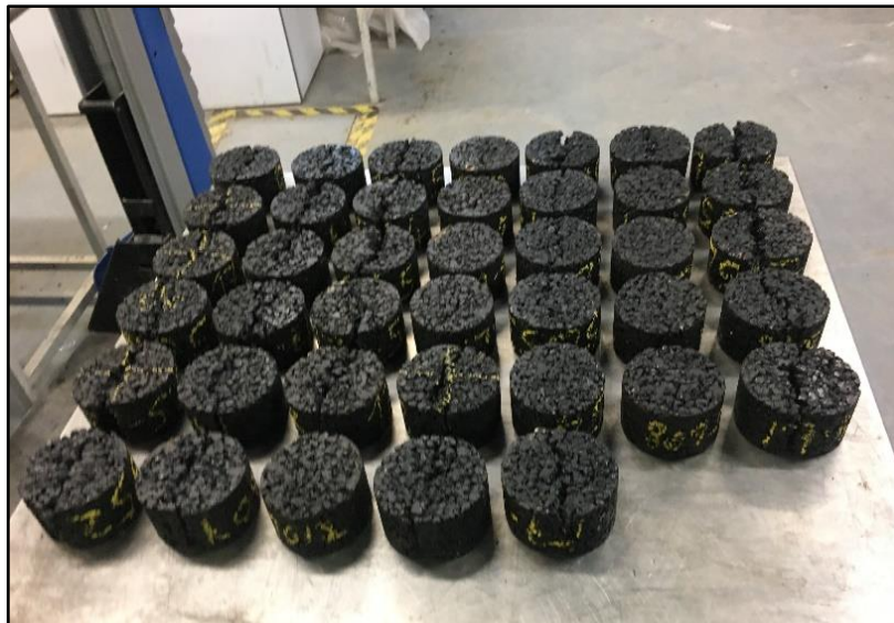
Figure 7.6. Appearance of samples after fatigue test.
