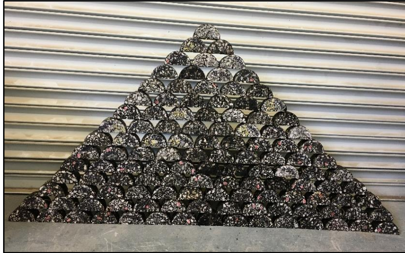
Figure 6.14. 3PB post-test appearance of aged samples.
