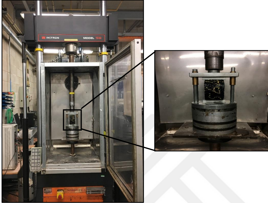
Figure 5.13. ITS test equipment.
