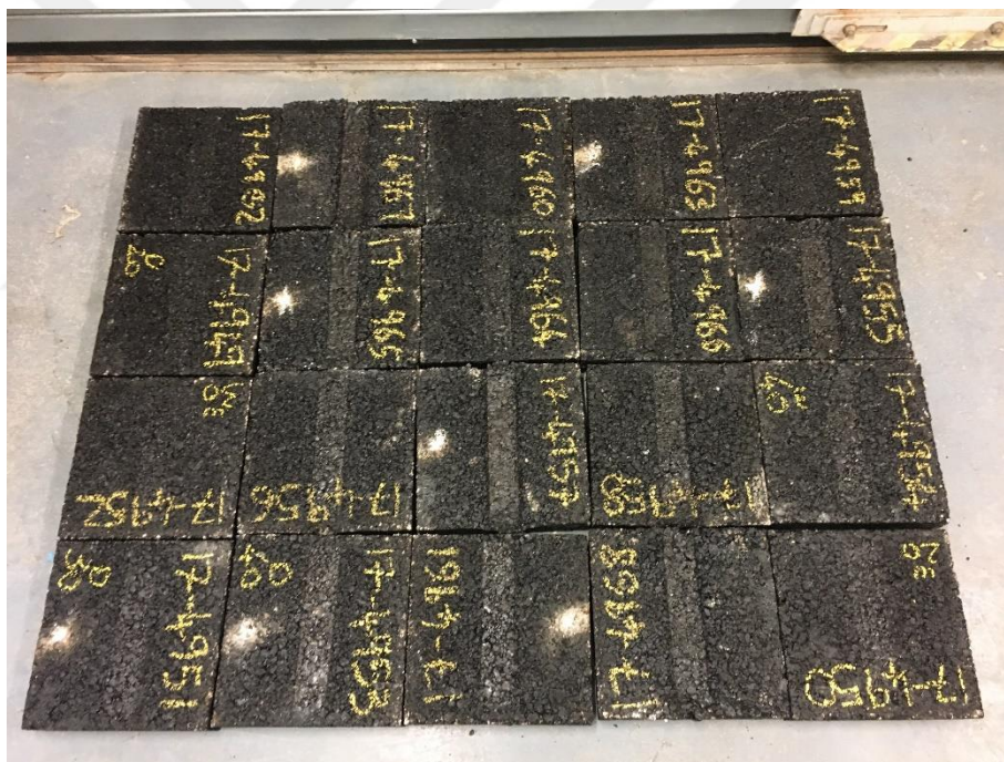
Figure 9.11. Samples after wheel tracking test.
