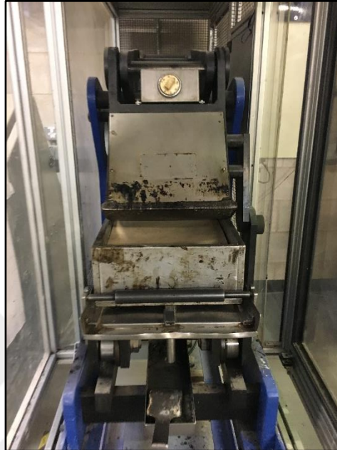
Figure 3.3. Slab roller compactor.
