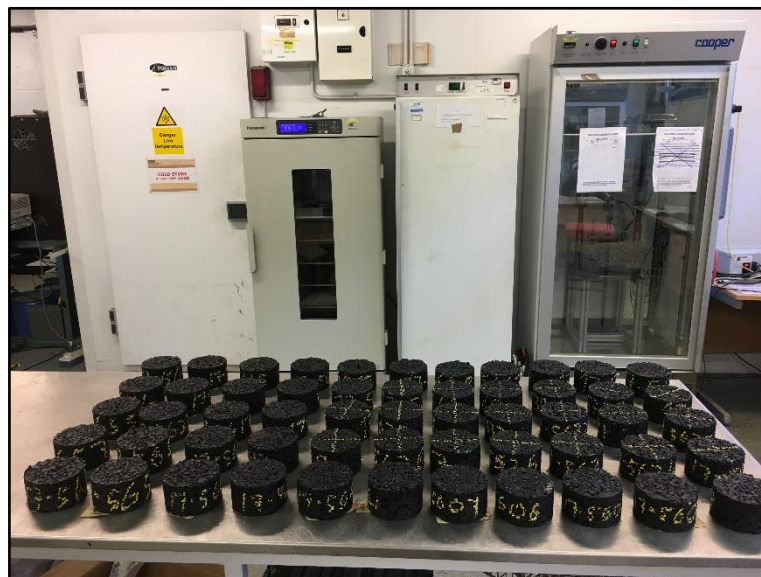
Figure 7.3. Appearance of SMA ITSM test specimens.
