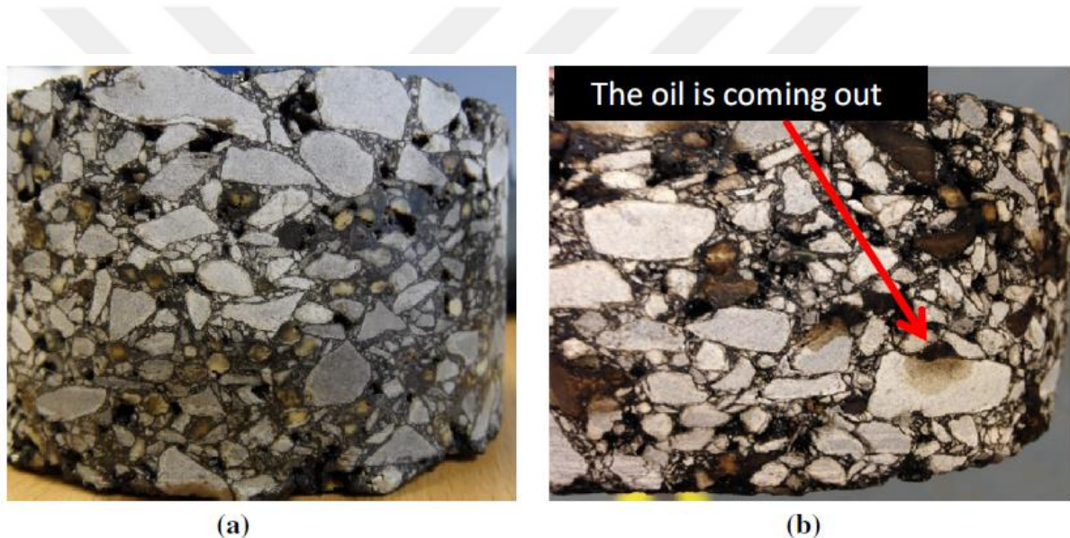
Figure 2.21. (a) Test sample before testing. (b) Test sample after testing, with capsules broken [54].
