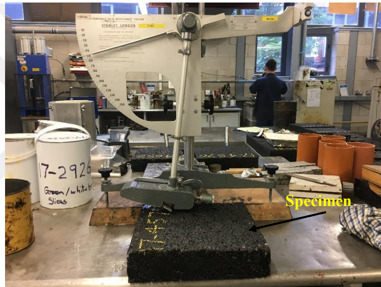
Figure 5.19. Skid test configuration.
