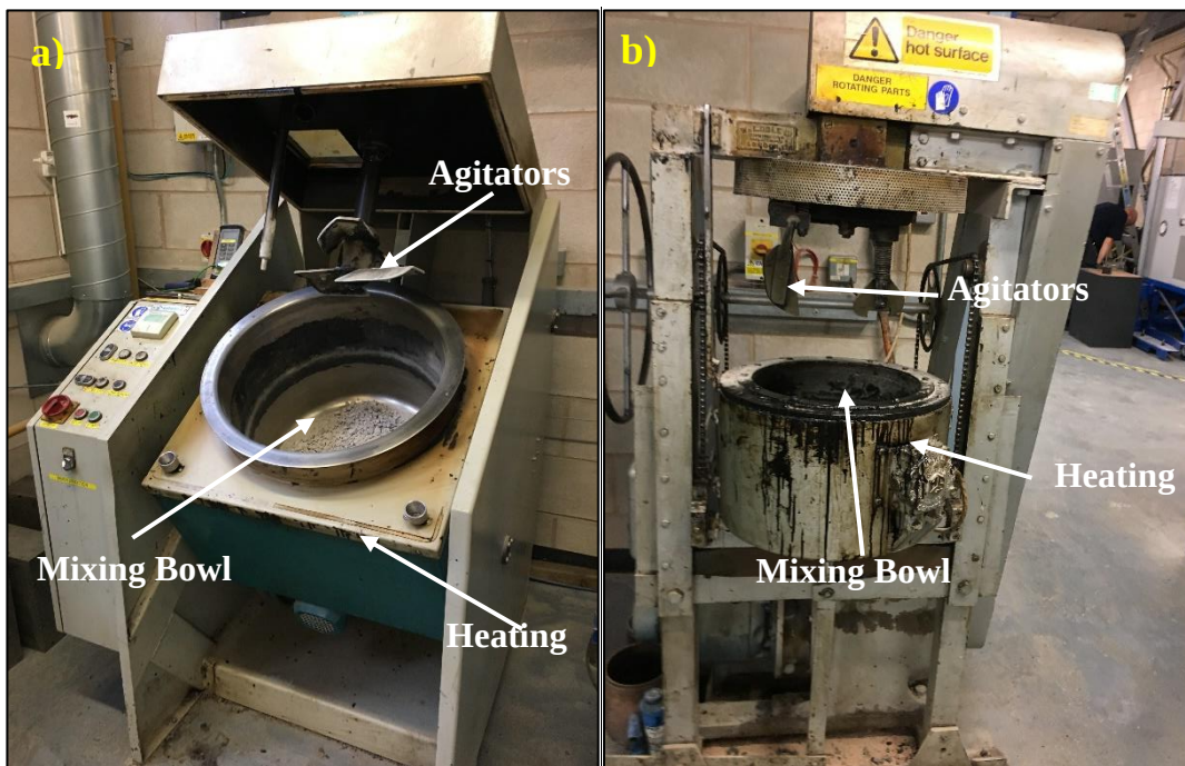
Figure 3.1. a)Inclined b) normal horizontal mixer.
