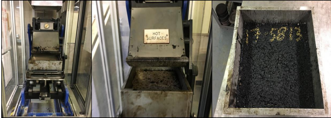
Figure 5.14. Roll press and sample preparation.
