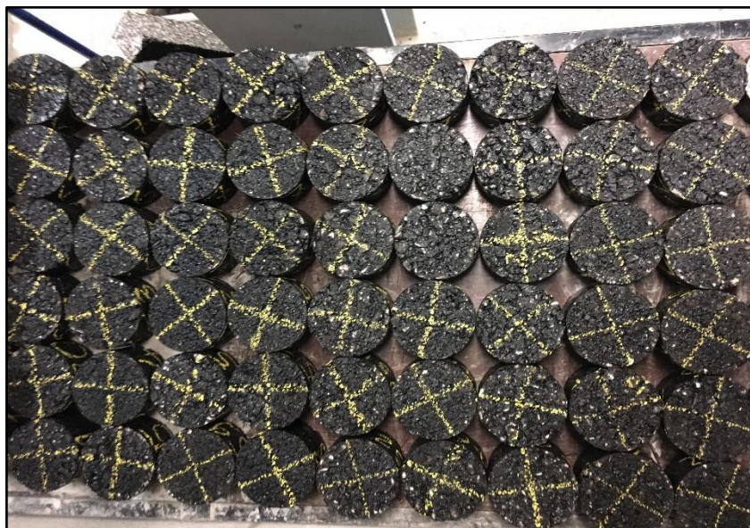
Figure 6.8. ITSM test samples.
