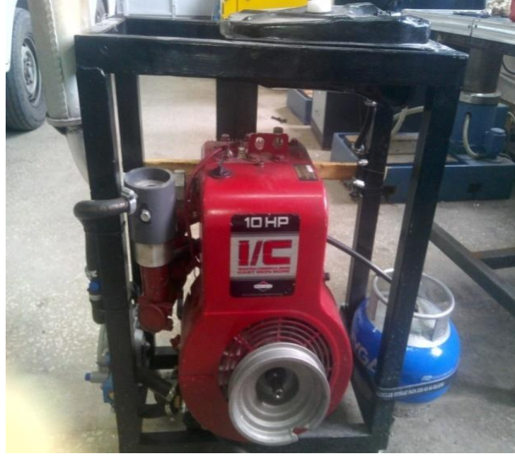
řekil 6.3. Briggs&Stratton I/C Cast Iron 10 HP LPG’li motor
