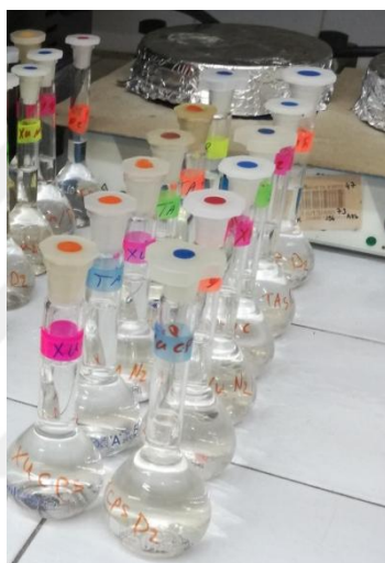
Figure 3.8. Soil Samples After Dry Digestion
