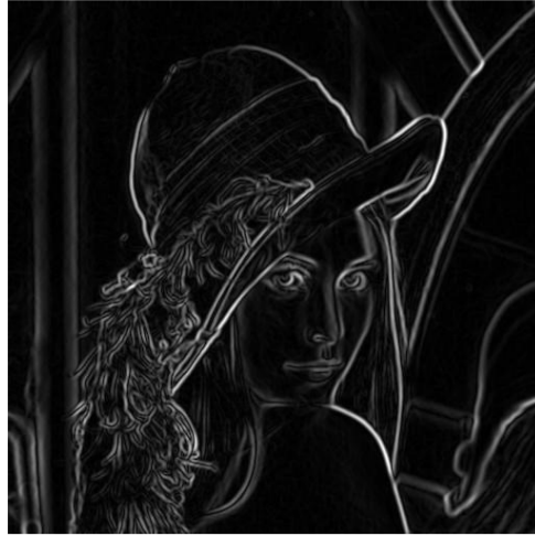
Figure 2.11 Intensity gradient calculation and edge direction finding process on an image.
