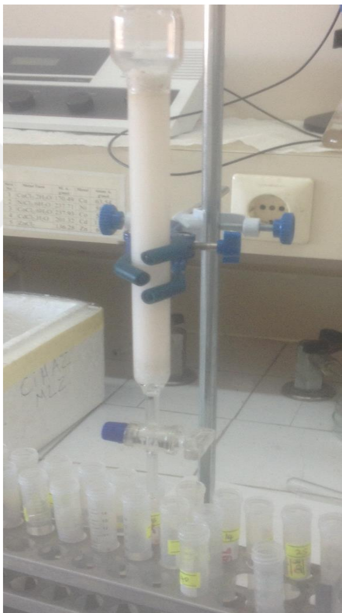
Figure 2.6. Showing Florisil column chromatographic set-up
