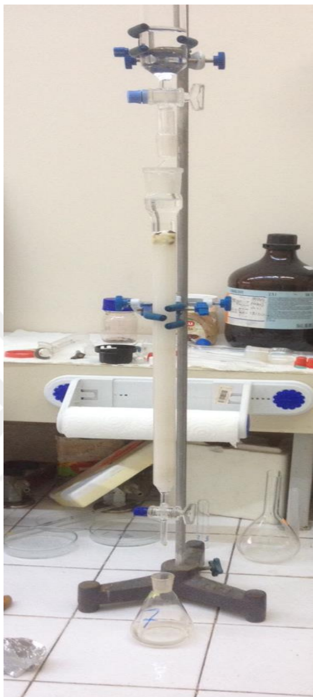
Figure 2.2. Showing silica gel column chromatographic set-up
