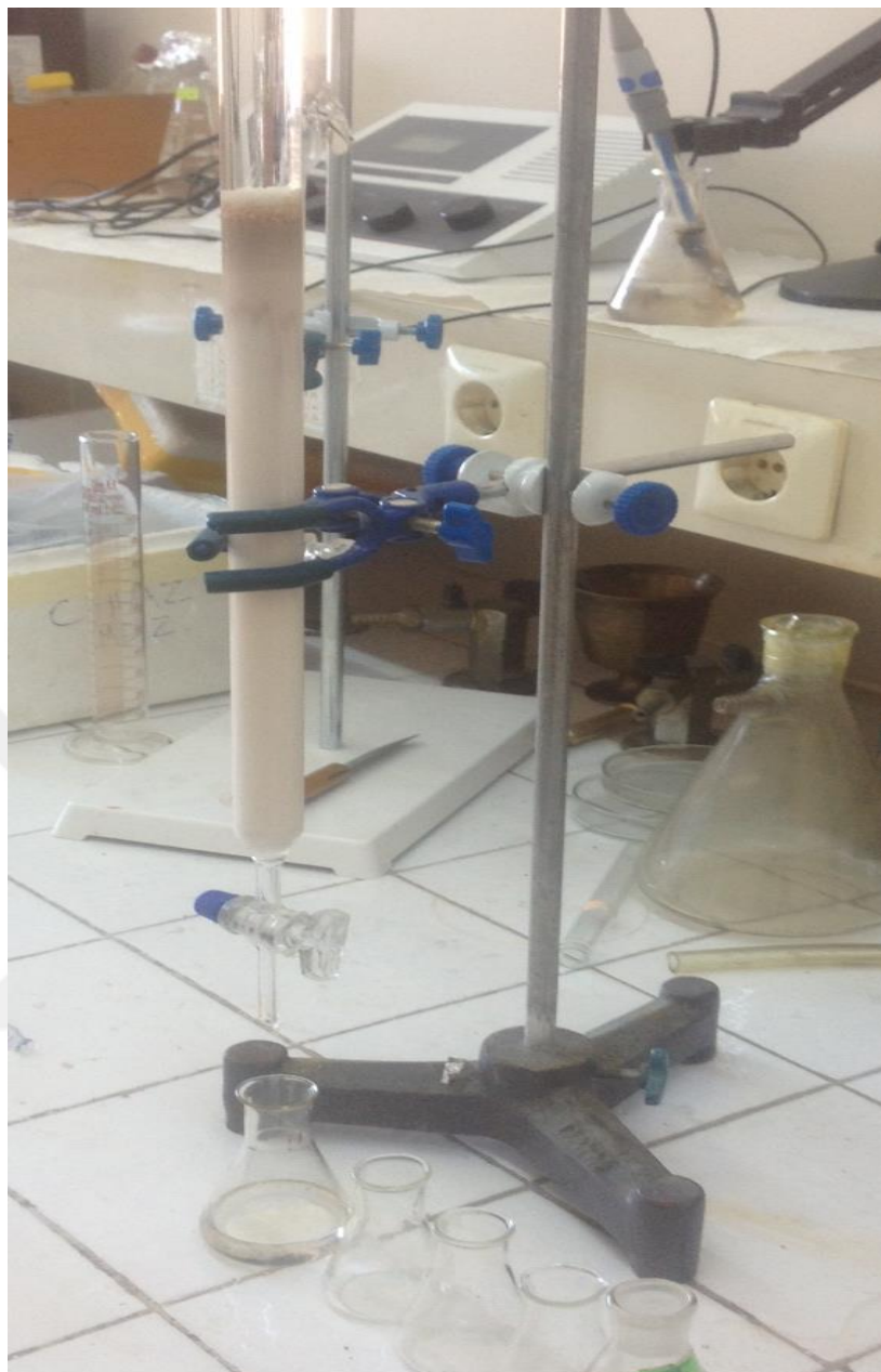
Figure 2.3. Showing Alumina column chromatographic set-up
