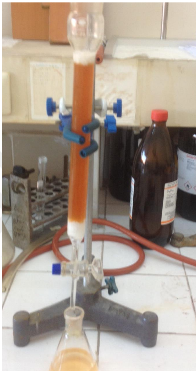
Figure 2.4. Showing Dowex cation exchange chromatographic set-up
