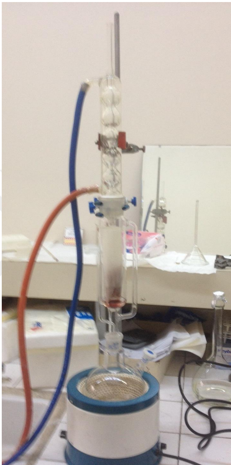
Figure 2.1. Showing soxhlet extraction setup used for solid liquid extraction of resveratrol from powdered grape seed.
