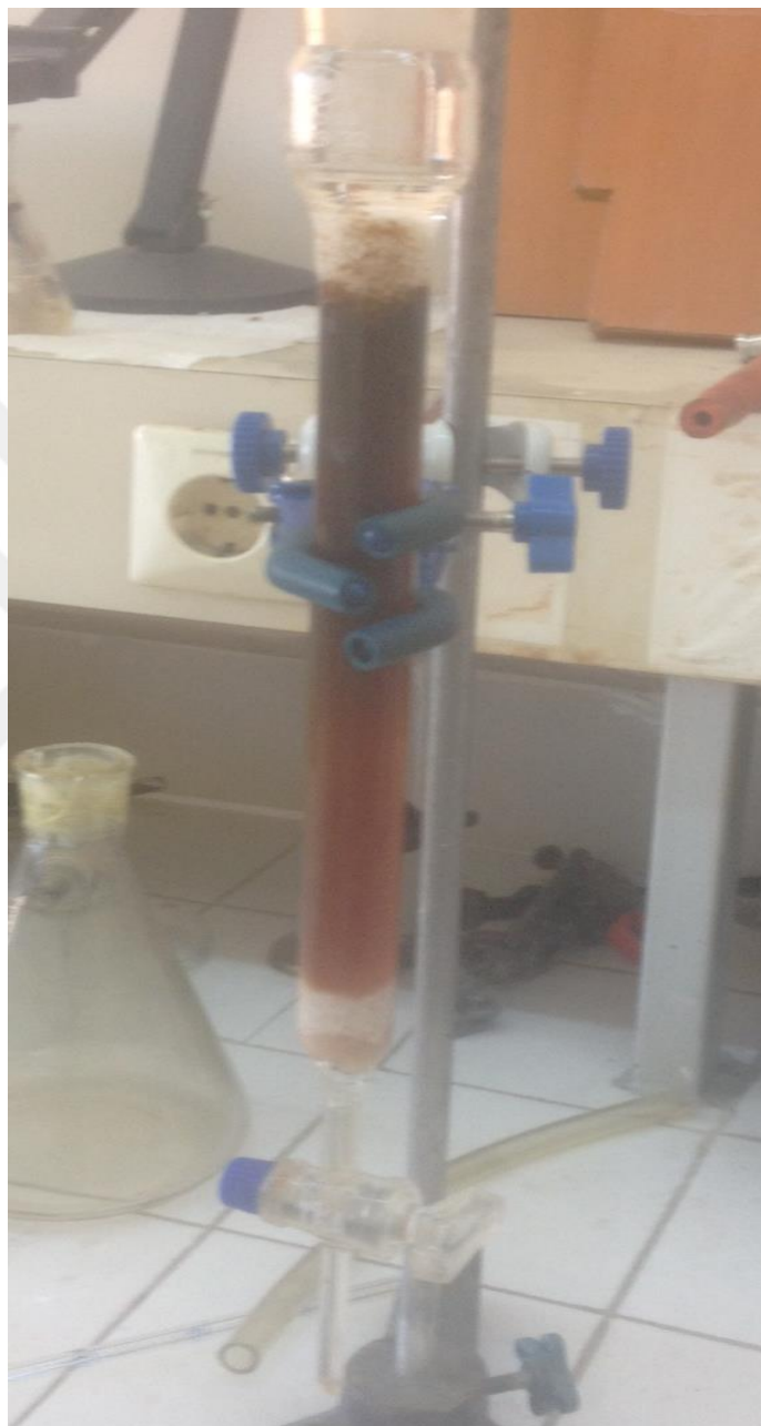
Figure 2.5. Showing Dowex anion exchange column chromatographic set-up
