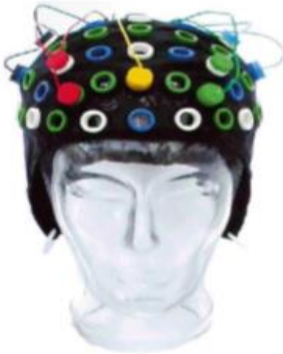
Figure 1.4: Non-Invasive BCI Electroencephalography (EEG) Electrodes Cap [8,9].
