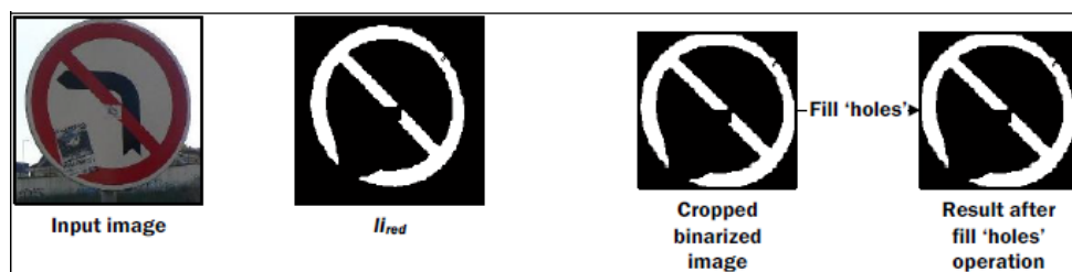
Figure 3.16: Problems on filling 'holes'
