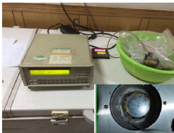
(c) Thermal conductivity test system
