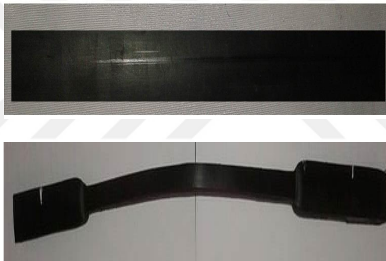
Figure 7.20. Tensile strip sample before and after testing.
