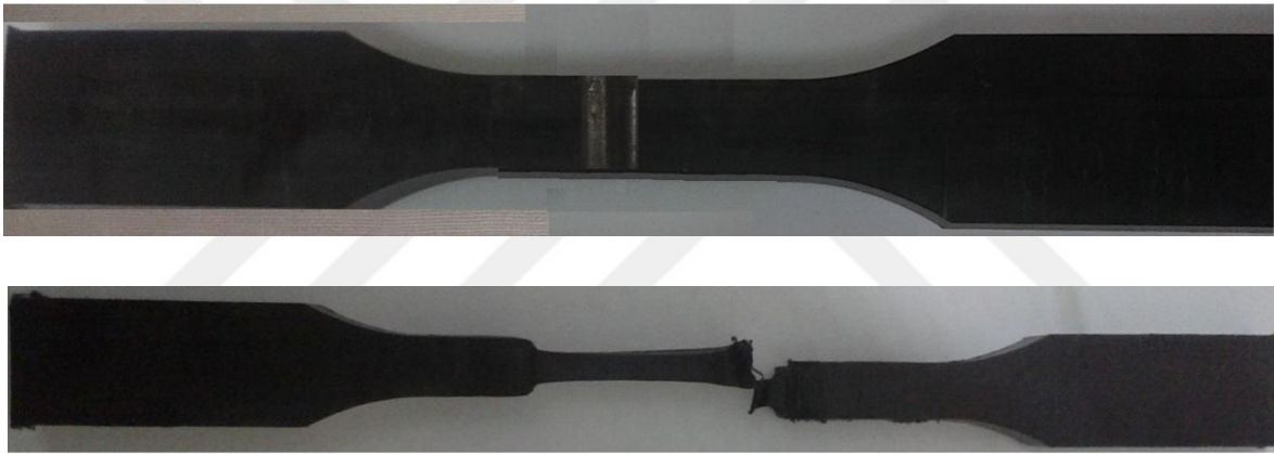
Figures 7.6. BFW tensile test sample before and after testing.
