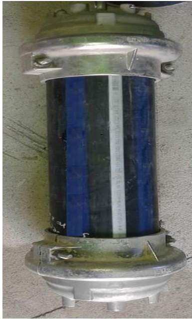
Figure 6.9. Sample for hydrostatic pressure test on HDPE pipe with end cap.
