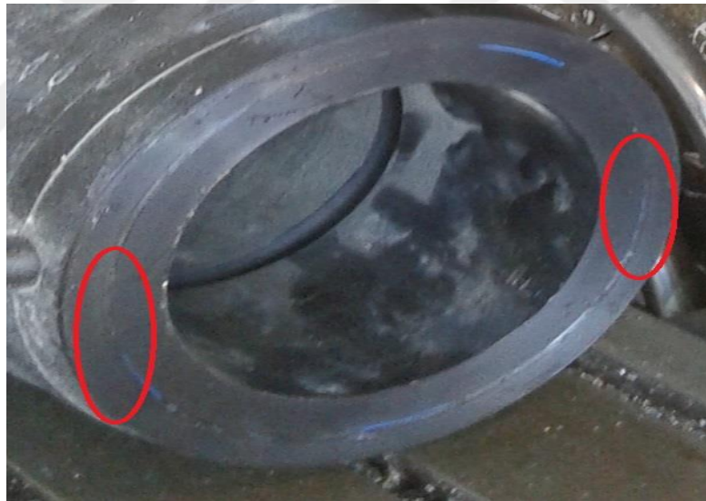
Figure 6.12. a) Sample of hydrostatic pressure test for EFW joint in HDPE and b) balancing distance between coupler and pipe by employing coupler alignment.
