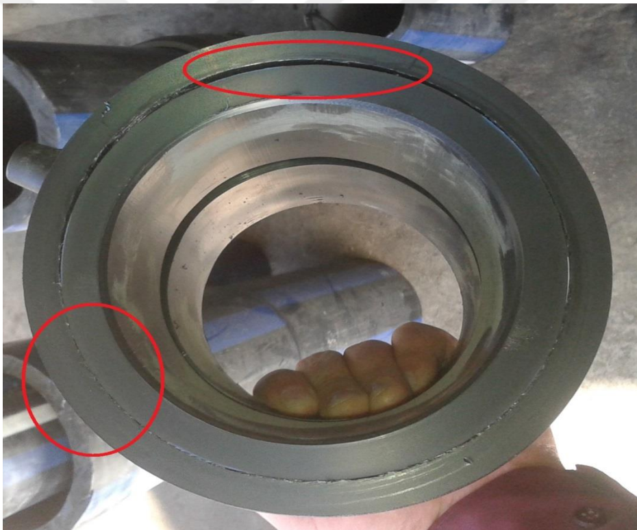
Figure 6.13. a) Sample of hydrostatic pressure test for EFW joint in HDPE and b) unbalancing distance between coupler and pipe after cooling.
